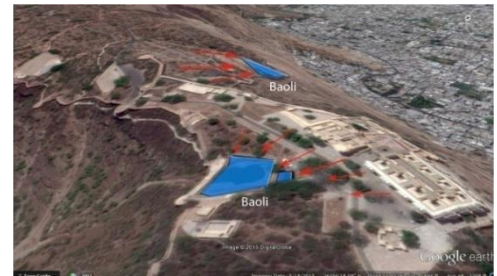
Fig 3.3.1: Nahargarh Fort Site drainage view (Aerial view of Nahargarh fort, depicting the slope of site and the location of Step wells on lower levels)
